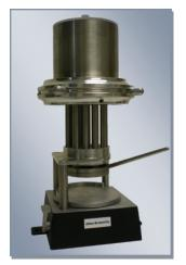
This stainless steel Peni Cylinder Dispenser holds 300+ cylinders and can dispense 4 or 6 cylinders. Cylinders are automatically and accurately dropped onto a Petri dish. Units may be modified for use with either glass or plastic Petri dishes.
